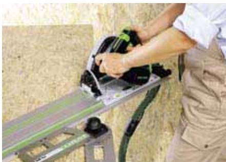
Simple transfer of angles to the workpiece with the combination bevel and guide rail.
